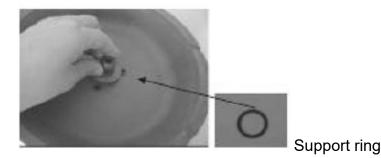
The support ring allows adjusting the sanding depth.
